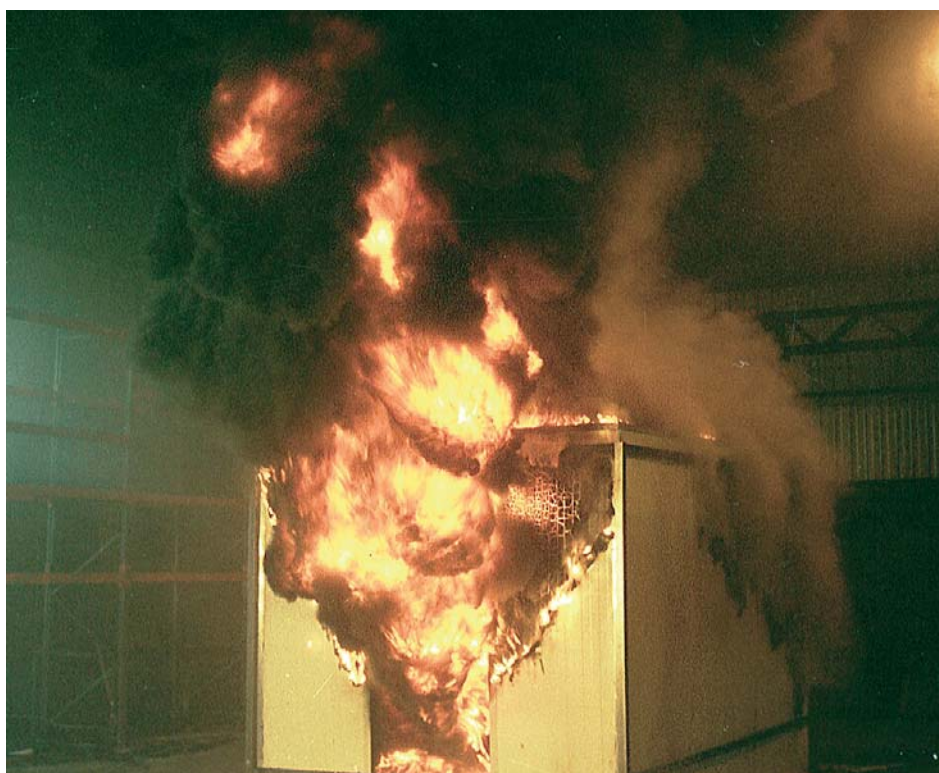
Flashover in a room constructed from sandwich panels in accordance with ISO 13784. Note the substantial smoke production.
